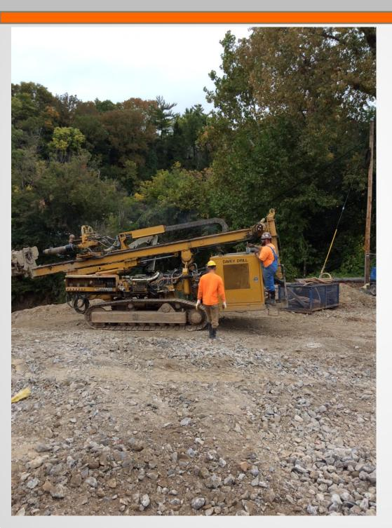
Diesel Driven, Hydraulic Machinery Requiring auxiliary Water and high pressure air to operate.
